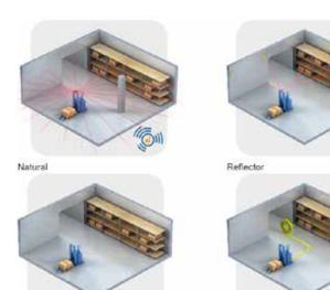
AGVs can be designed to utilize a number of navigation technologies available in the market today. Depending on the complexity of a facility, our engineers will recommend the best possible navigation method for a system. The illustration to the left, shows some of the more popular navigation methods today. Other methods include bar-code and inductive wire.
