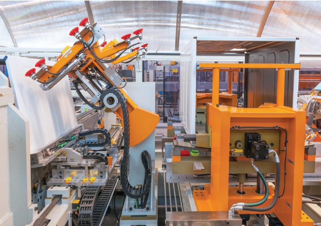
Top loading washer cabinet production line. One of two now in service, achieving high volume production to exacting quality requirements, and manufactured to the very latest safety standards.
