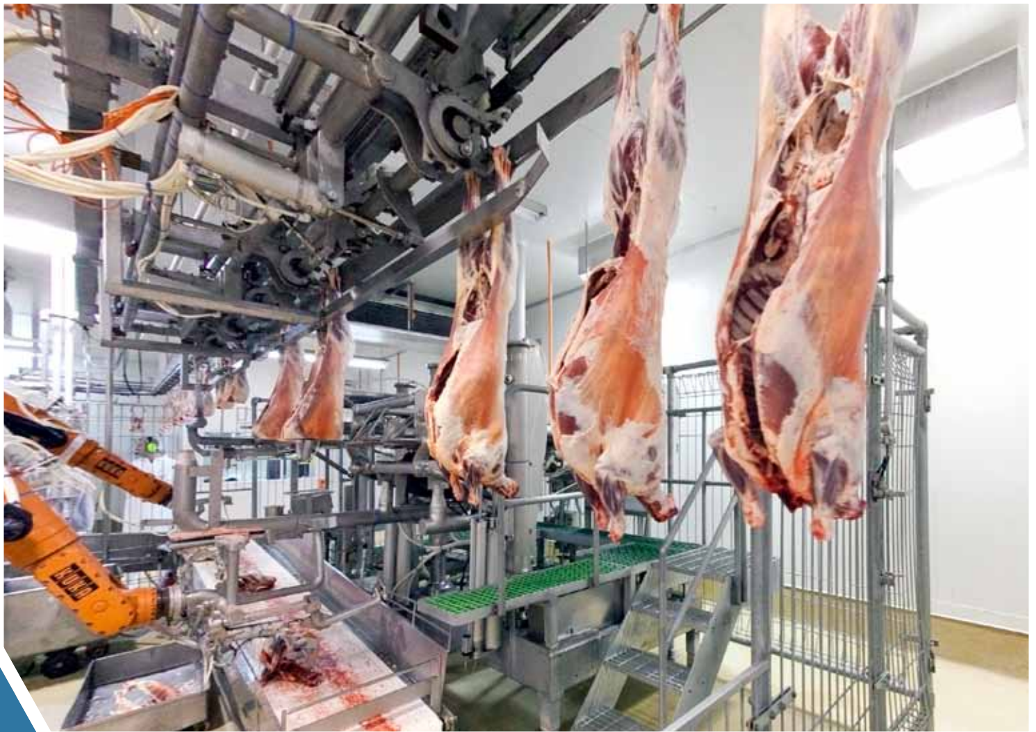
ABOVE: Automated primal cutting system at Silver Fern Farms' Finegand plant.
