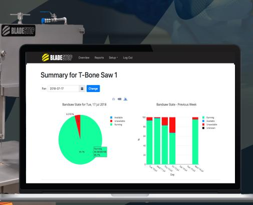
BladeStop Bandsaws equipped with Bladestop Connect gives real time and historical data showing productivity and event information. Data is easily accessed from any local intranet connected device.
